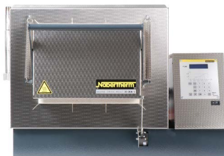
Figure 16: Furnace for Ash Content RDC 169
