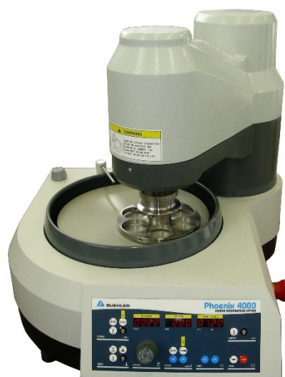
Figure 12: Test Arrangement for the Determination of the Abrasion (RDC 191)
