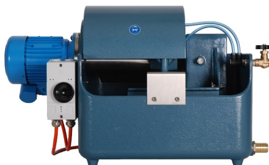
Figure 2: Example of a Diamond Wheel Saw (RDC 148)
